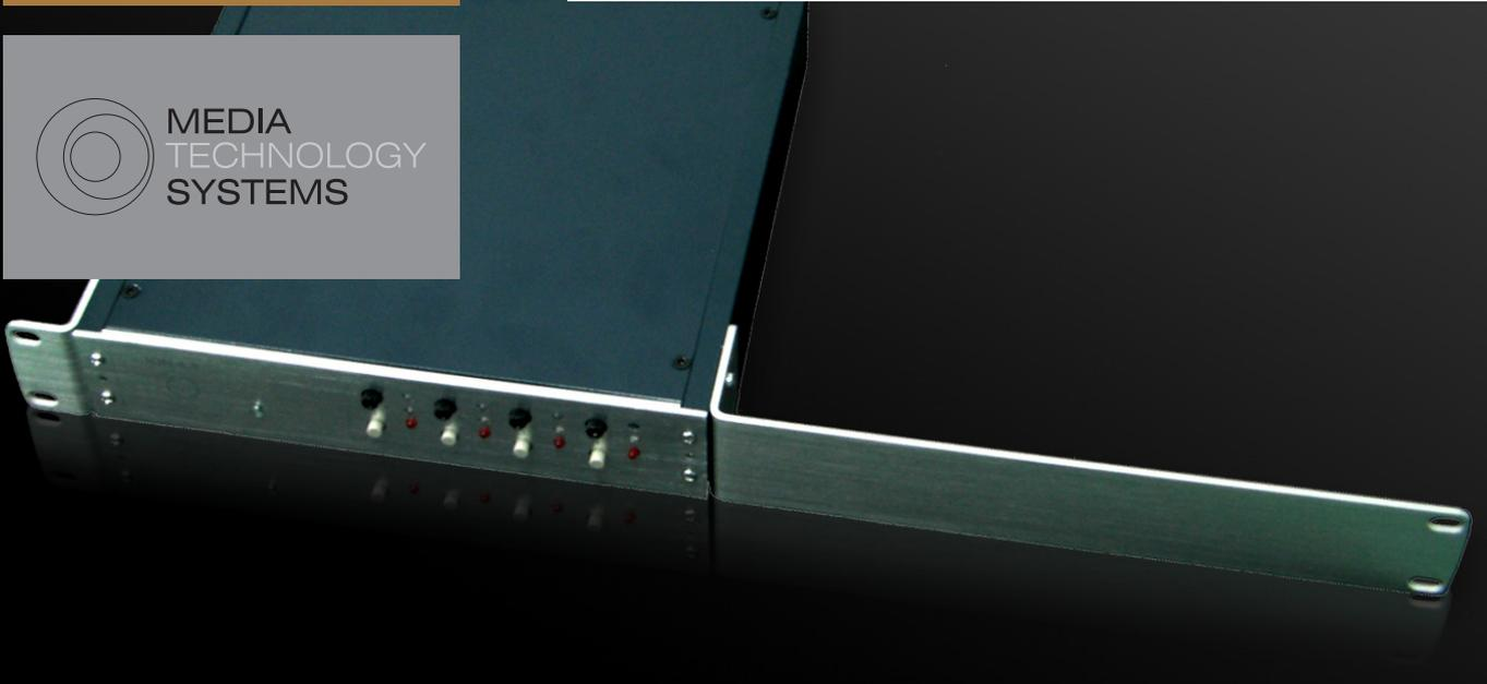
The Media Technology Systems ION4.4 is a CobraNet® 1/2 width 1U rack mount configuration with 4 analog mic/line inputs and 4 analog outputs. In addition, the chassis can be vertically mounted on a wall, riser or upside-down under a table. This mounting flexibility allows the installer to convert the analog audio to a LAN data stream in remote locations.
