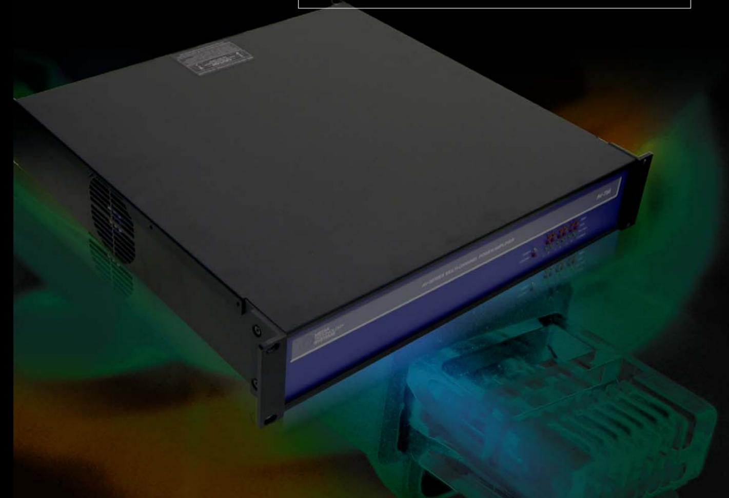
The AV series amplifiers employ a Class D output topology for maximum efficiency and does not require high volume, forced fan cooling even with the amplifier running into clip on all channels. In addition, the switch mode power supply (SMPS) incorporates power factor correction (PFC) to comply with incoming legislation and minimize noise pollution of the electrical supply.
