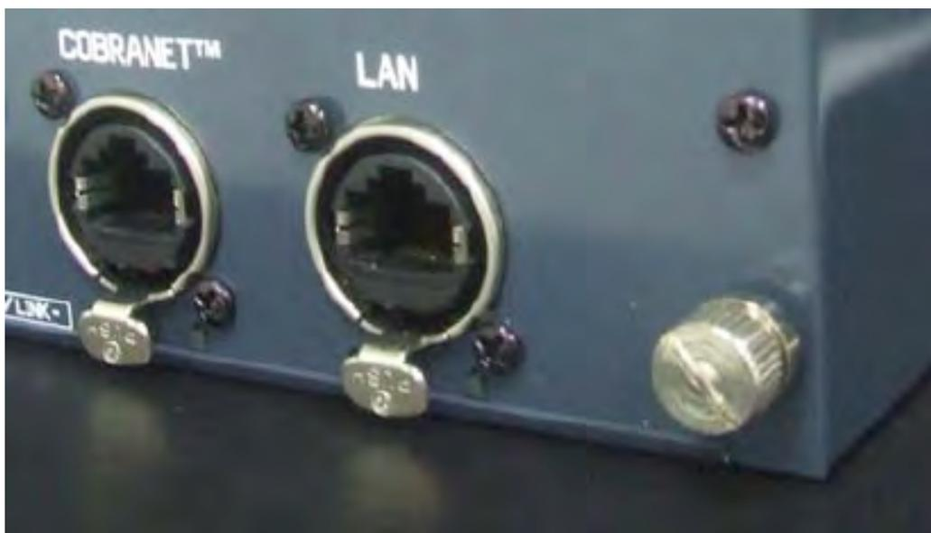
Figure 3-6: Rear chassis panel showing ground pin
